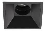
Square black downlight. DEEP is a series of recessed luminaires designed for lighting retail and work spaces. The 15° version is ideal for spot lighting. With a heat temperature of 3000K, this downlight allows warm, comfortable atmospheres to be created. The Honeycomb diffuser allows a light projection with less glare.
